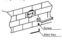
Finally,hang the main body to thrust on thewall, tighten screws with spanner,confirm installment is reliable
