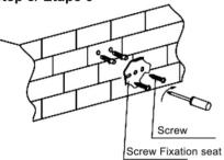
Use Cross screwdriver to tighten screw and fix bracket on the wall.
