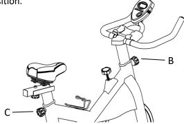
To adjust the height of the handlebar, first loosen the adjustment knob M1 (B) and pull it outward. Then, move the handlebar upward or downward, release the adjustment knob into an adjustment hole in the handlebar, and firmly tighten the adjustment knob.
